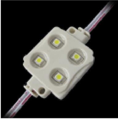
Waterproof SMD 4LEDs Module adopts 4 pcs of SMD LED as its luminous body, this product has good ability, wide beaming angle, and perfect design. ABS Engineering Plastic Housing glued with epoxy makes the product wholly waterproof (IP 65).
